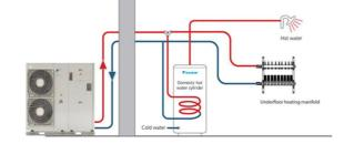
A Split-Bloc heat pump (SBHP) will provide the dwellings with heating and hot water. Hot water is provided indirectly via an integrated hot water storage cylinder. There is an indoor unit and an outdoor unit when a Split-Bloc heat pump is installed with connecting refrigerant pipework entering the dwellings. The integrated hot water cylinder offers energy efficiency benefits over the Monobloc heat pump.
